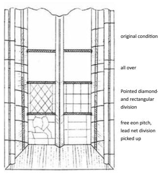
Test panels of this window side in float glass
